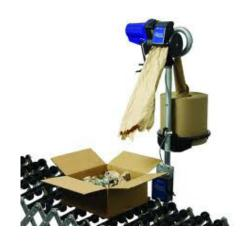
"The machine, which delivers crumpled paper from rollstock at speeds of up to 150 inches per second, establishes a new performance standard for this category."
